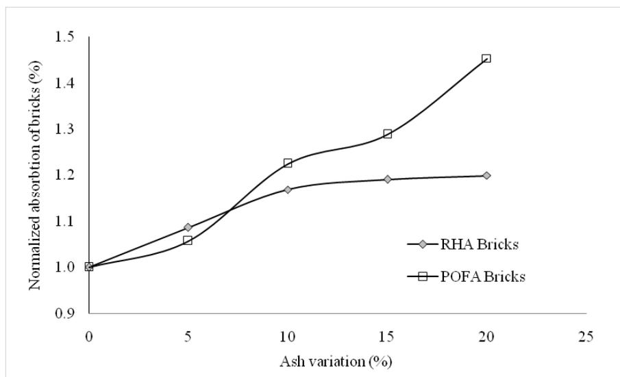
Figure 1. The absorption of RHA and POFA bricks.
