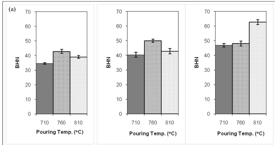
Figure 4. Hardness value with different pouring temperature on (a) Al-1.37Zn-1.19Si; (b) Al-1.66Si-1.35Zn; and (c) Al-2.81Zn-2.6Si alloys.
